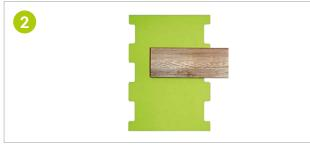
2. Decide the direction in which your flooring will be laid and install GREEN LIGNIN at a 90° angle to the long side of the floor boards.
