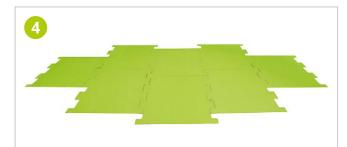
4. Lay the GREEN LIGNIN sheets loosely together on the subfloor with the sheets offset from each other by half a width. If necessary, fix the plates with adhesive tape.
